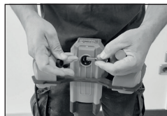
Replacement of carbon brushes.
